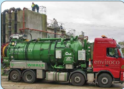
"Given that we service a number of remote locations on land, not to mention the high level of offshore work that we undertake, the Kaiser-Whale represents a truly cost-effective solution as the water it recycles can be used for jetting. As you can imagine, this delivers significant operational, environmental and economic benefits."
