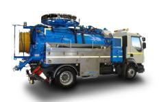
Sewer cleaning jet-vac with continuous water recycling
