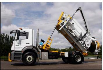
A demountable Whale Medium Volume Combination equipped with Econ's Quick Change Body (QCB) system.
