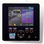
Capable of interfacing with the manufacturer's chassis and CANbus system, the controller allows a number of new key features, including diagnostics. It has an in-built flexibility to
