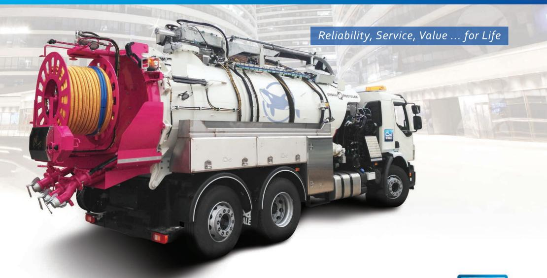
Sewer cleaning jet-vac with continuous water recycling
